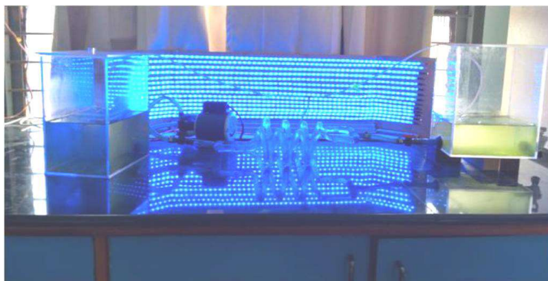
Fig. 2: Designed and fabricated PBR with LED light source.
